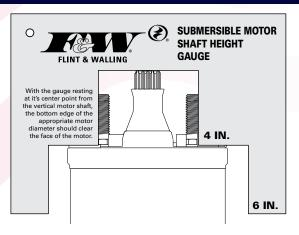
With the 024456 gauge resting at it's center point from the vertical motor shaft, the bottom edge of the appropriate motor diameter should clear the face of the motor.
